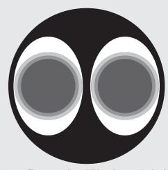
The white area illustrates the additional space in the borehole when upsizing to a larger, oval-shaped dimension. As shown, there is still sufficient room for a smooth installation.
